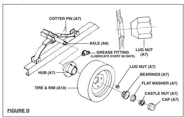
10. Carefully slide the Hubs (A7) over the Spindles at each end of the Axle (A6). Insert the Bearings (A7) and the Flat Washer (A7) on the Spindles. Screw a Castle Nut
